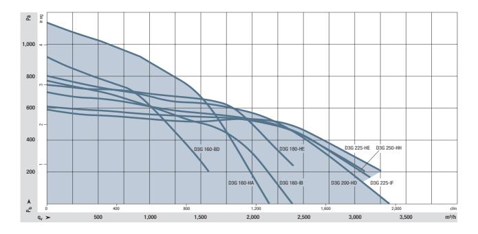
Fan power measurements are carried out on state-of-the-art chamber test rigs. The entire fan unit, consisting of motor, control electronics, and impeller, is measured at varying load states. This ensures that we obtain reliable data, and that you can count on these values being reached when selecting a fan. There are therefore no nasty surprises in store when starting up the fans.
