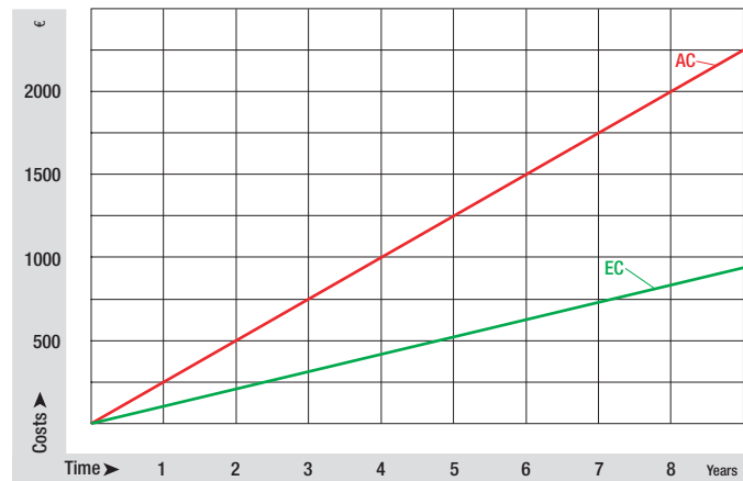
Figure: Operating costs over time at 0.10 EUR/kWh
